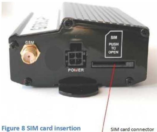
Figure 8 SIM card insertion
